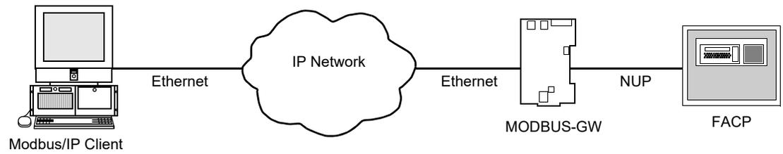
**Figure 1.1 Single Panel Architecture**
