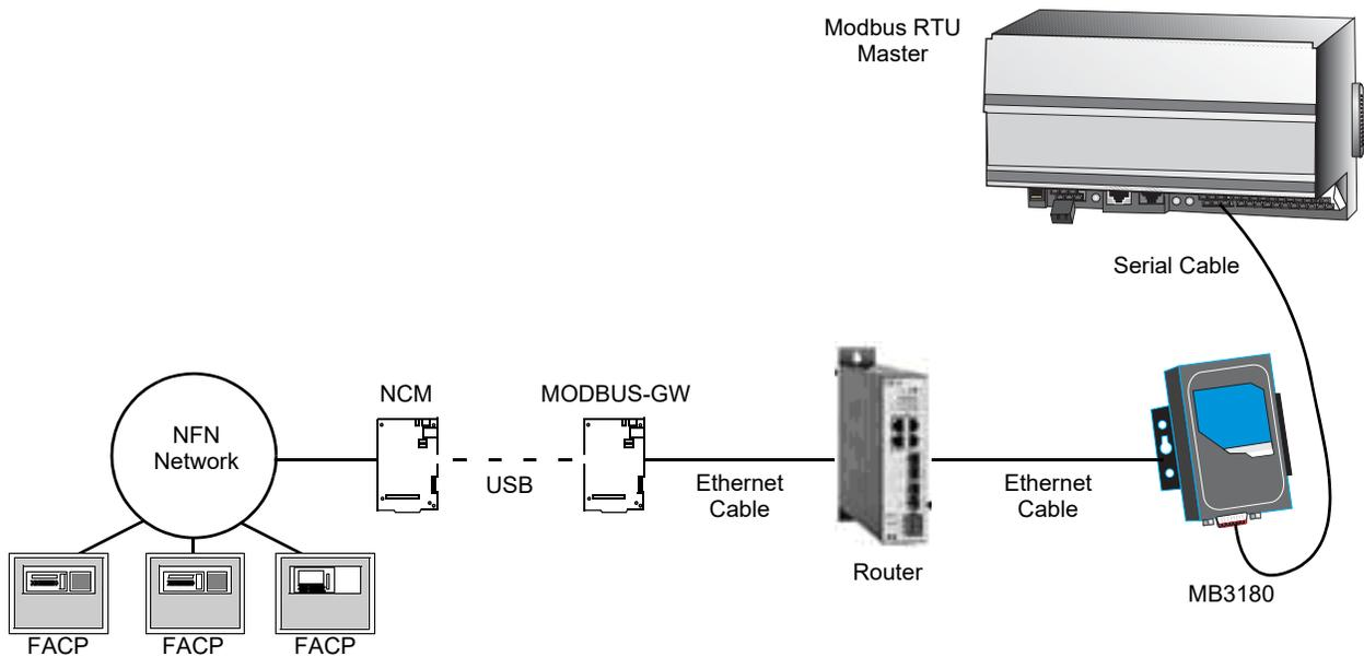
**Figure F.3 Connection Through a Router**
