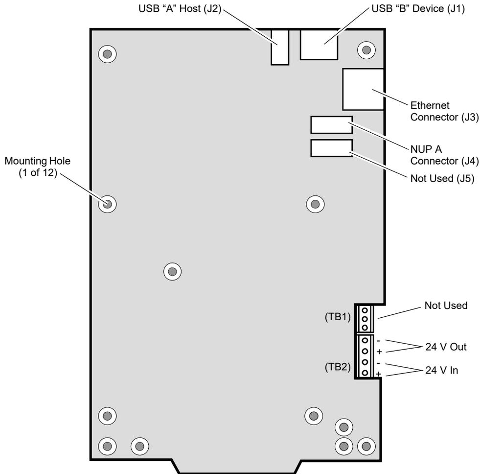
Figure 2.5 MODBUS-GW Connections
