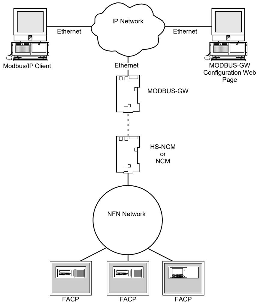
**Figure 1.2 NFN Network Architecture**
