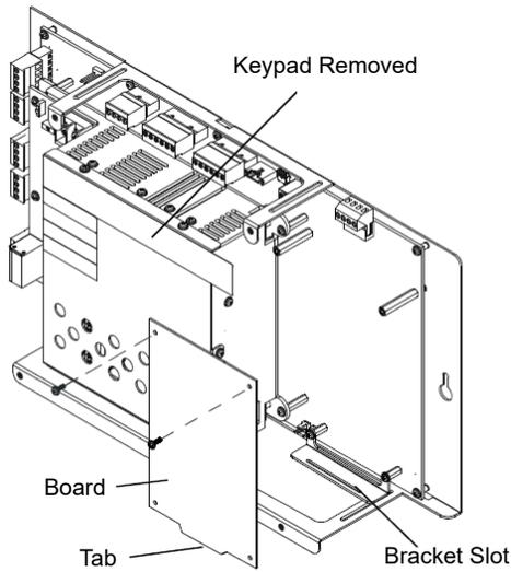
Install bracket on 1/2" standoffs. Place the board's tab in the bracket slot and screw the board to the top of the standoffs. May be stacked in front of or behind another board using standoffs of adequate length to clear the rear board.
