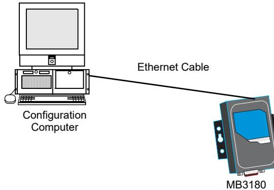
**Figure F.1 Connect a Configuration Computer**
