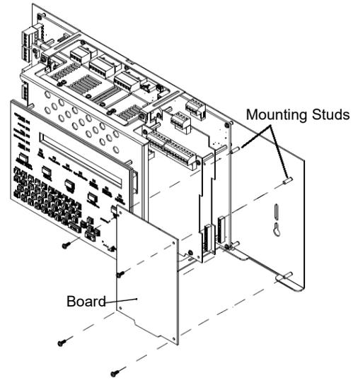
Mount in 4th column of the NFS2-640 Series chassis. Mount chassis to backbox before installing the board in rear position. May be mounted in front of another board using standoffs of adequate length to clear the rear board.
