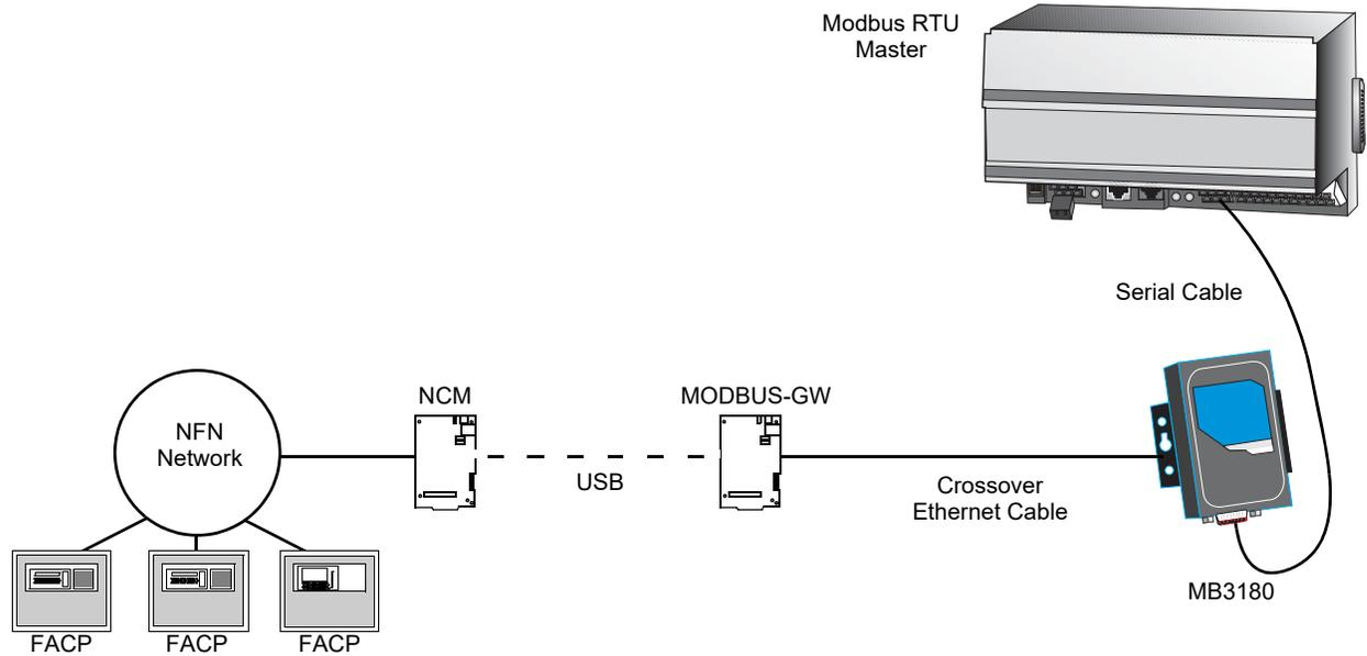
**Figure F.2 Connection Through Crossover Ethernet Cable**
