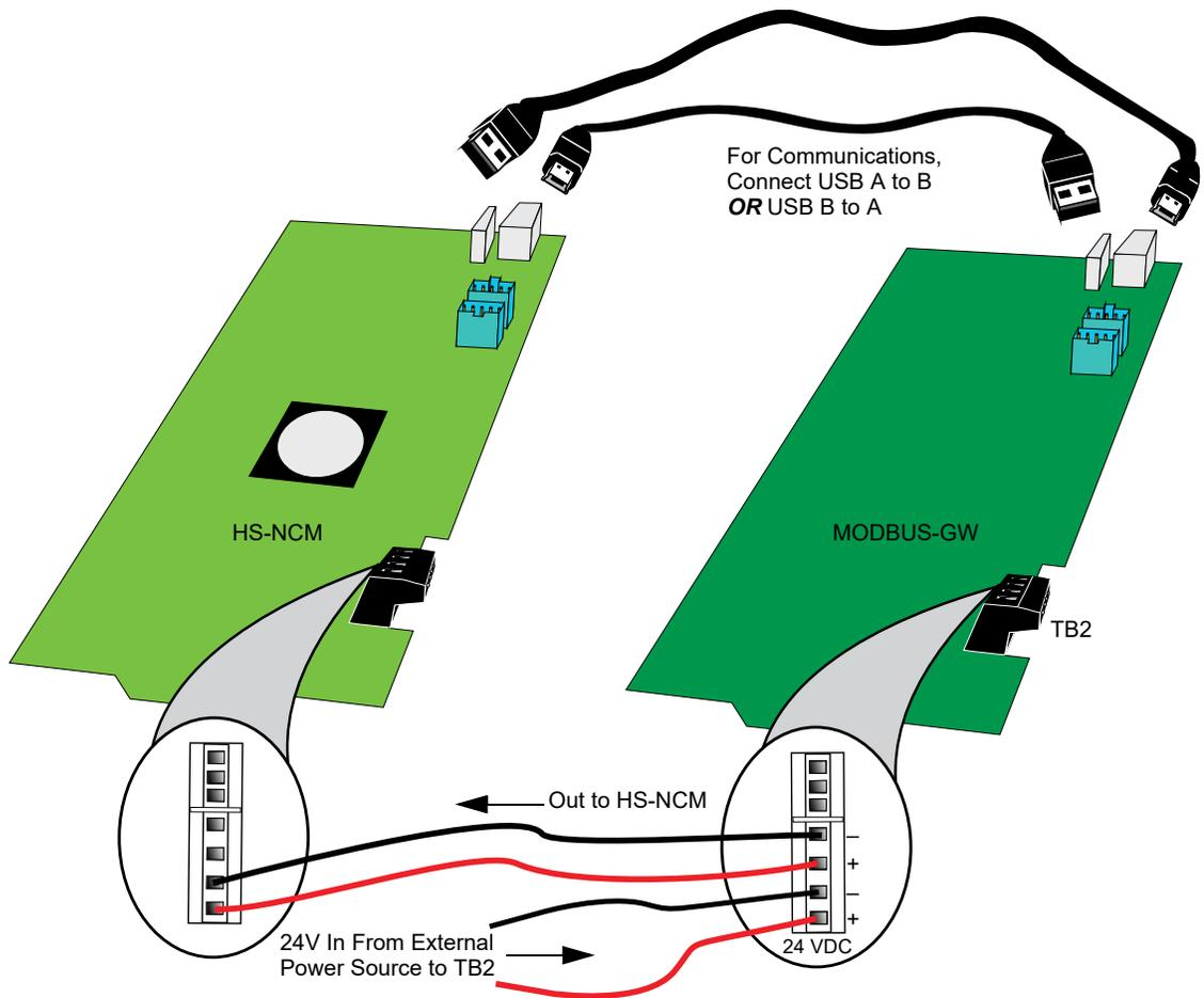
Figure 2.8 Routing Power and Communication to an HS-NCM
